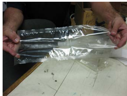
OEP plastic air bladder used in damper/diffuser
