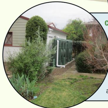
**Rooftop downspout disconnection.** By directing rooftop runoff onto vegetated areas, you can direct the water to areas where it will be useful rather than being conveyed to the stormwater system where it may cause harm or overload the pipe system.
