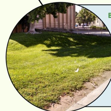
**Vegetated swales** are shallow, open grass channels that can be an alternative to traditional curbs and gutters. Vegetated swales are designed to convey runoff while providing limited pollutant removal by sedimentation and horizontal filtration through vegetation.
