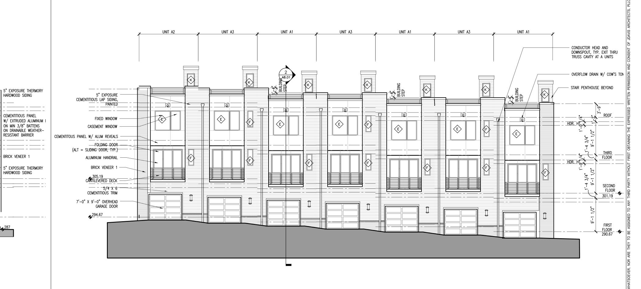
BUILDING 5 SIDE (WEST) ELEVATION SCALE: 1/8" = 1'-0"
