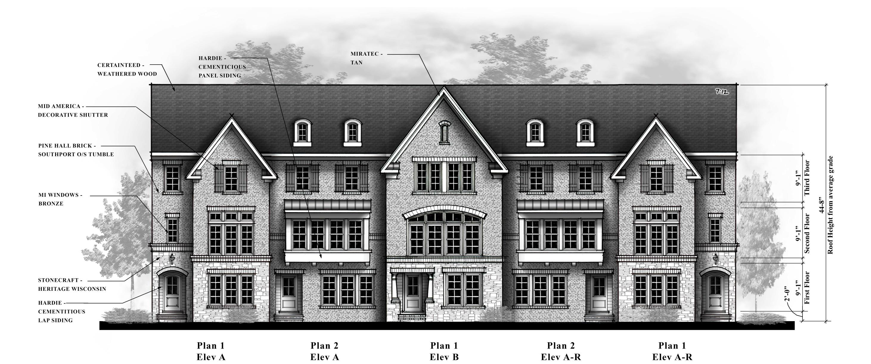
Front Elevation  $\frac{\text{Front Elevation}}{3/16\text{"}=1\text{'}-0\text{"}}$
