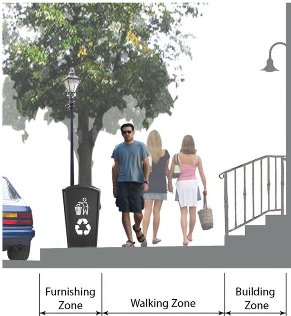
Photo 27. A sidewalk comprised of three zones is typical in urban areas.
