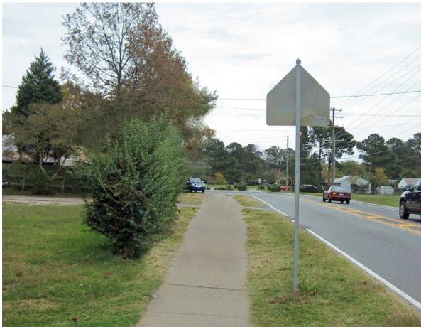
Photo 28. Shrubbery can reduce the space for pedestrians to travel along a sidewalk.
