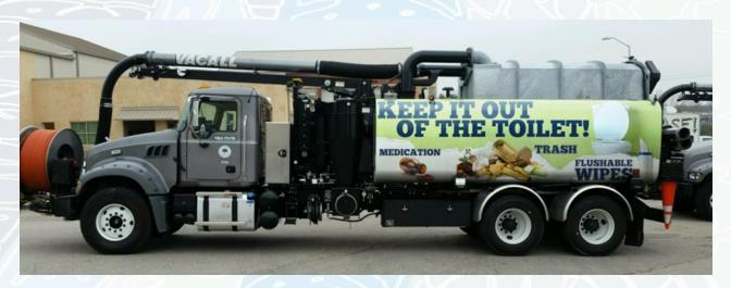
While an important part of avoiding sanitary sewer overflows is reducing the introduction of inappropriate materials into the sewer collection system, the Department also operates a fleet of flusher trucks which help keep the sewer lines clear of blockages. With over 2,500 miles of sewer lines to maintain, you've probably seen one of our 15 flush trucks driving in our service area, which includes the surrounding communities of Wake Forest, Zebulon, Wendell, Rolesville, Garner, and Knightdale.
