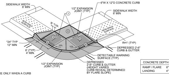
NOTE: \* USE SMALL FLARE ONLY WHEN A CURB WOULD DIRECTLY CONFLICT WITH APPROACHING VEHICLE TURNING MOVEMENTS.
